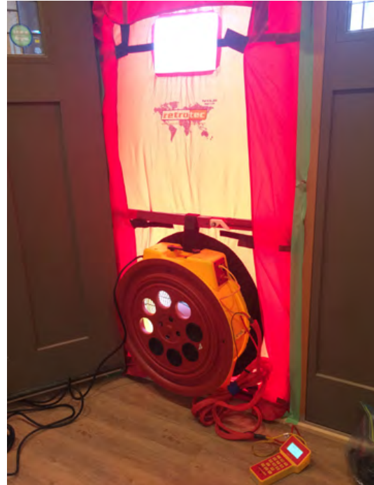
Figure 8: Blower door test in action
